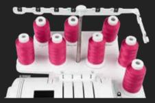
Rolled Hem. Flatlock. or Cover Stitch: The Aspire's basic configuration, featuring a maximum of five threads, allows for a wide range of stitch combinations and decorative effects. Additionally, the optional Spool Holder enables sewing with up to eight threads.
