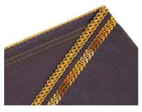
7-thread Expressive Stitch consisting of a Triple Cover Stitch combined with a 3-thread Narrow Overlock
